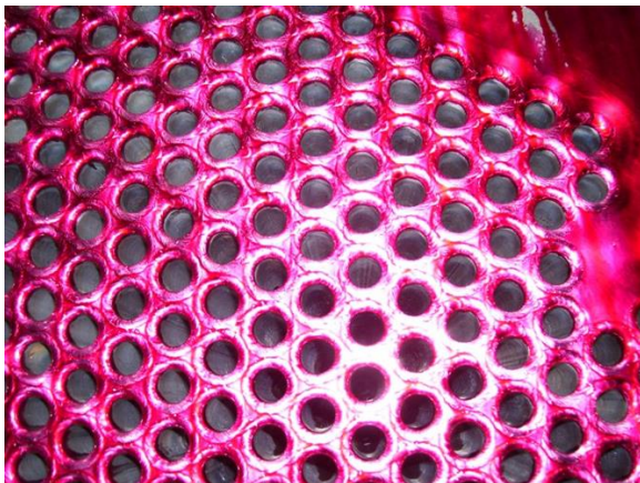
Fig 13 – DPT of Tube to Tubesheet Welds Fig 14 – Soap bubble solution applied to test welds
