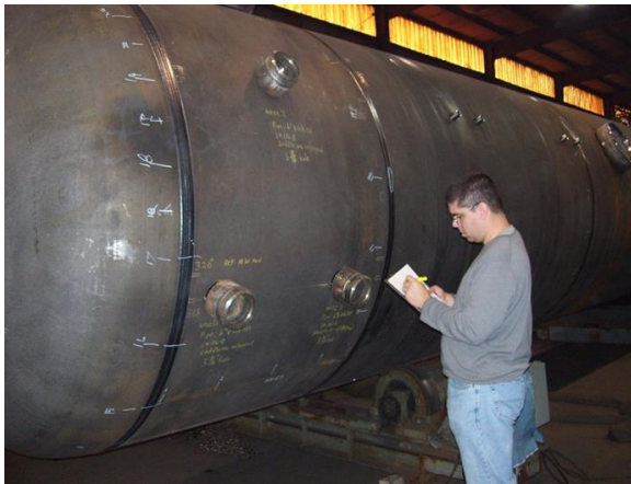
Fig 10 – Verification of Nozzle Placement
