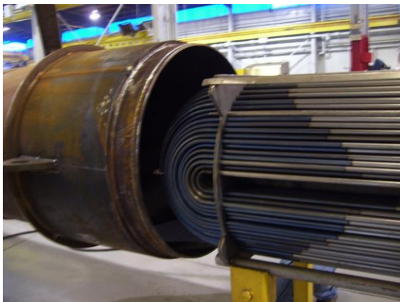
Fig 12 – Bundle insertion into Shell
