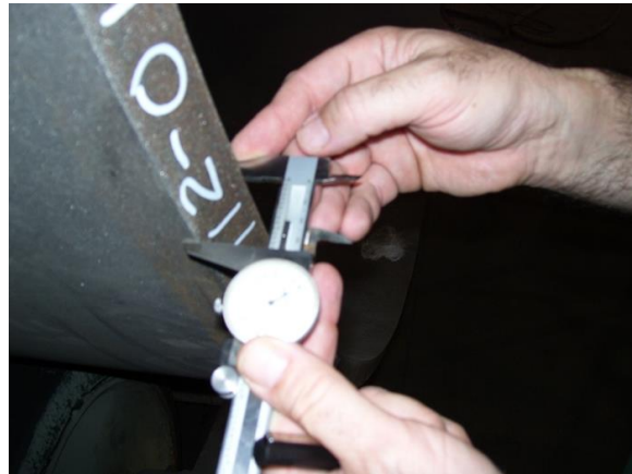
Fig 11 – Check of Shell Thickness
