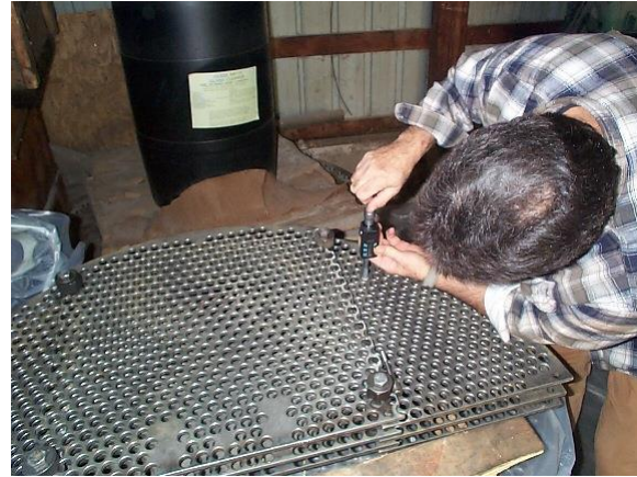
Fig 6 – Dimensional check of baffle holes
