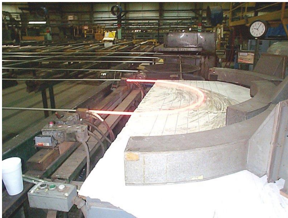
Fig 1 – Stress Relief of a U-bend
