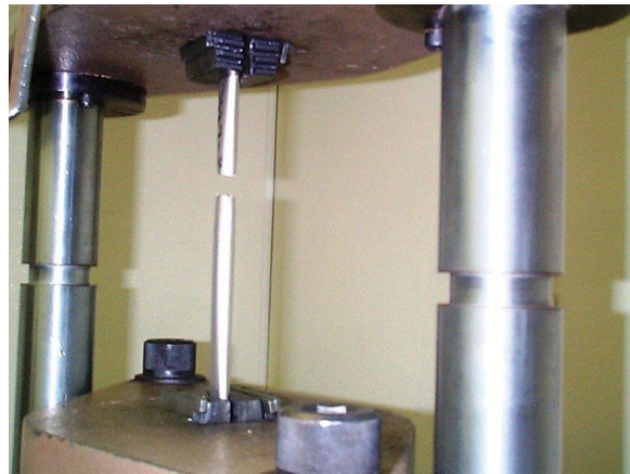
Fig 2 – Tensile Test of Tube Sample
